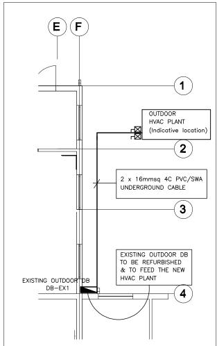
PART GROUND FLOOR SHOWING POWER SUPPLY RETICULATION TO NEW OUTDOOR HVAC PLANT
