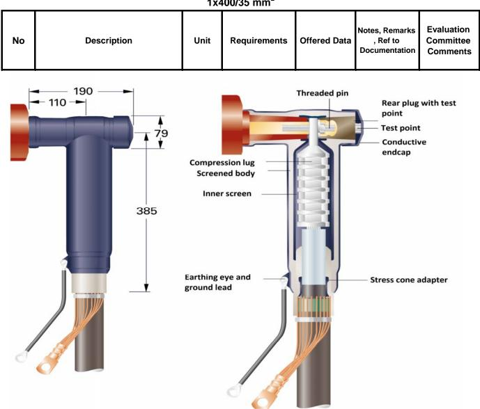
630A , 24 kv Indoor Screened Separable Termination Kit for 12/20 kv XLPE Cable  $1x400/35 \text{ mm}^2$
