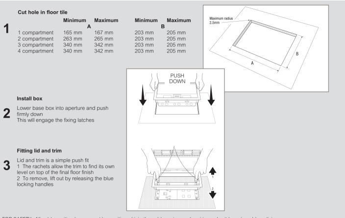
FOR SAFETY : All cables exiting boxes must be positioned into the cable routers on box trim and exit box via cable outlets Lid and lid handle must always be placed in the closed positions When using metal lid and trims, the lifting device at the centre of the lid is not to be used as a cable exit
