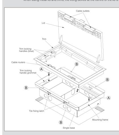
Opening lid to an angle of 30° and lifting upwards will detach lid from trim. Inserting lid into the opposite side of trim will change direction of the lid
