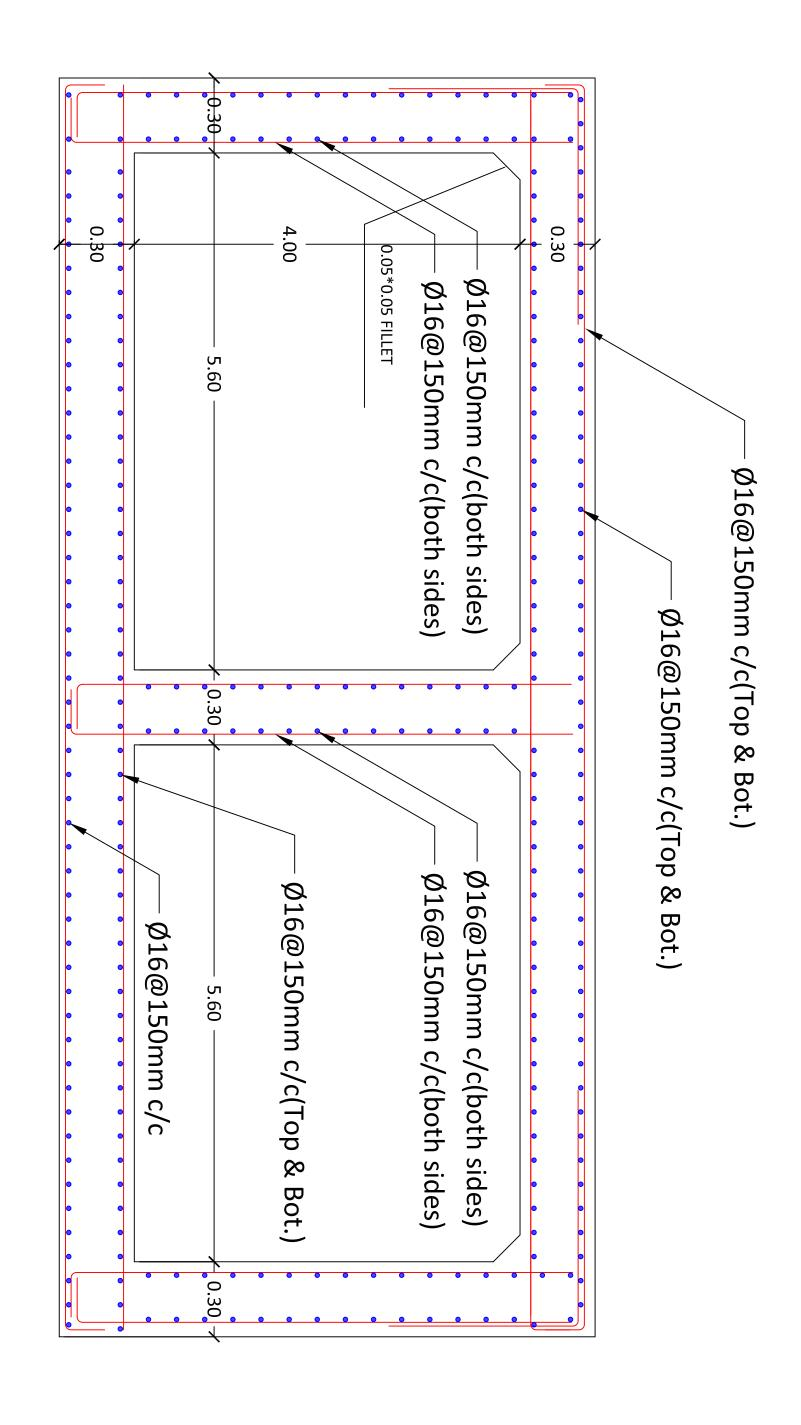
Detail of double cell box culvert5.6x4.0m
