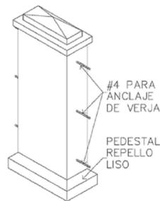
DETALLE DE PILASTRA EN BARANDAS DE CONCRETO CON BALAUSTRÉS - NIVEL 000
