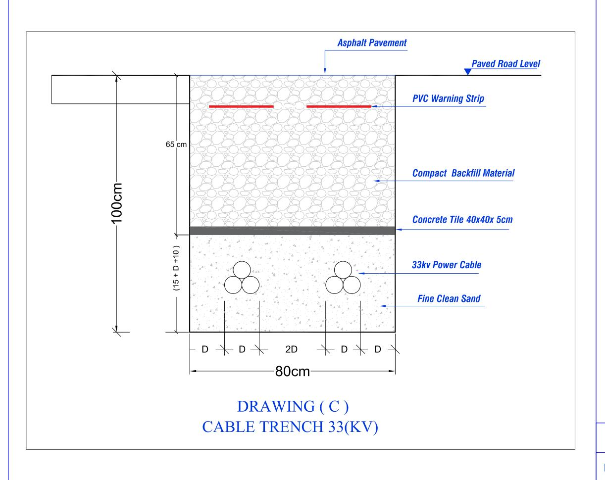
Trench width W = 6DSingle core cable diameter = dD=2d=110mm (approximately) W = 6x110 = 660mm The Trench should be not less than 660mm and not more than 800mm
