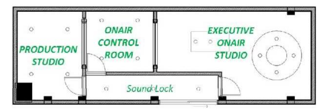
Executive Onair studio will contain minimal equipment, like microphones, monitor speakers, a computer with internet access and operator telephone hybrid. All the other controls will be located
