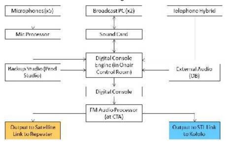
The onair digital console engine should have a minimum of 12 inputs with VGA connection point and software to enable control or programming by technical operator. All connections to the system should be digital or have digital converters to input into the console engine. Output from the console engine to FM Audio processor should also be by digital connection.
