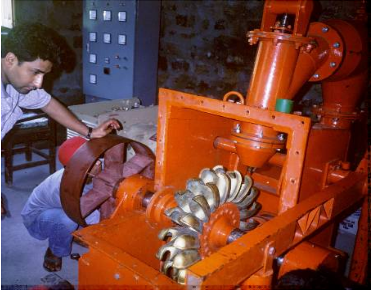
Double Jets Pelton Turbine with Magnetic Jet Deflector
