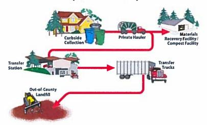
Within this context, three solid waste transfer stations will be constructed in Kırıkhan and Yayladağ districts of Hatay and Hilvan district of Şanlıurfa. Stations will be mainly composed of administrative/weigh building, waste loading bunker, waste spilling platform, ramps, intra-site roads and landscaping. System of transfer station will be "push pit", waste collection trucks dump their loads directly to a trailer.
