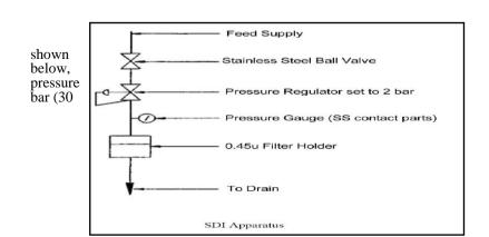
1. Assemble the apparatus as in the figure and set the regulator to 2 psig)
