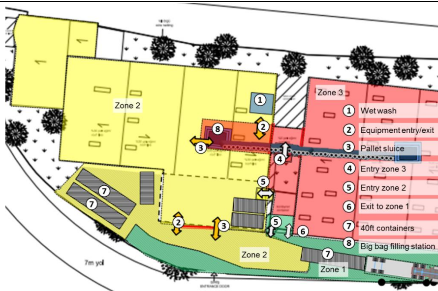
Figure 4: Recommended Phase 4 (Main (Primary) POPs Waste Stockpile Elimination) On-site Zoning Configuration ((North is to the left of the picture. Warehouse 6, excluded from picture is classified as Zone 3) 15
