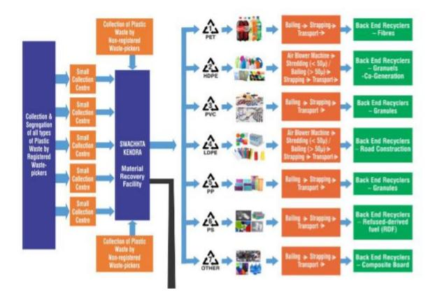
In the **Figure I**, it clearly defines the schematic diagram of how the collection and processing of the plastic waste will be done. Consideration will also be given to development of innovative methods for mechanical recycling/upcycling; including improved segregation into 07 different categories of plastic wastes (as authorised SW Mgt. rules 2016, as shown in the above figure 1) to improve the quality of the recycled materials and better pricing for the segregated plastics.
