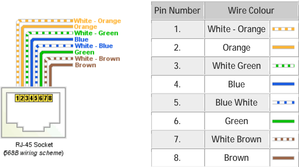
Fig2. EIA/TIA 568B Network Wiring Scheme
