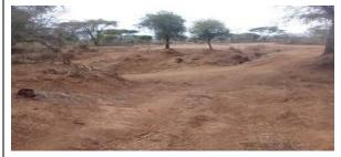
Figure 32: seasonal Stream; no drainage structure
