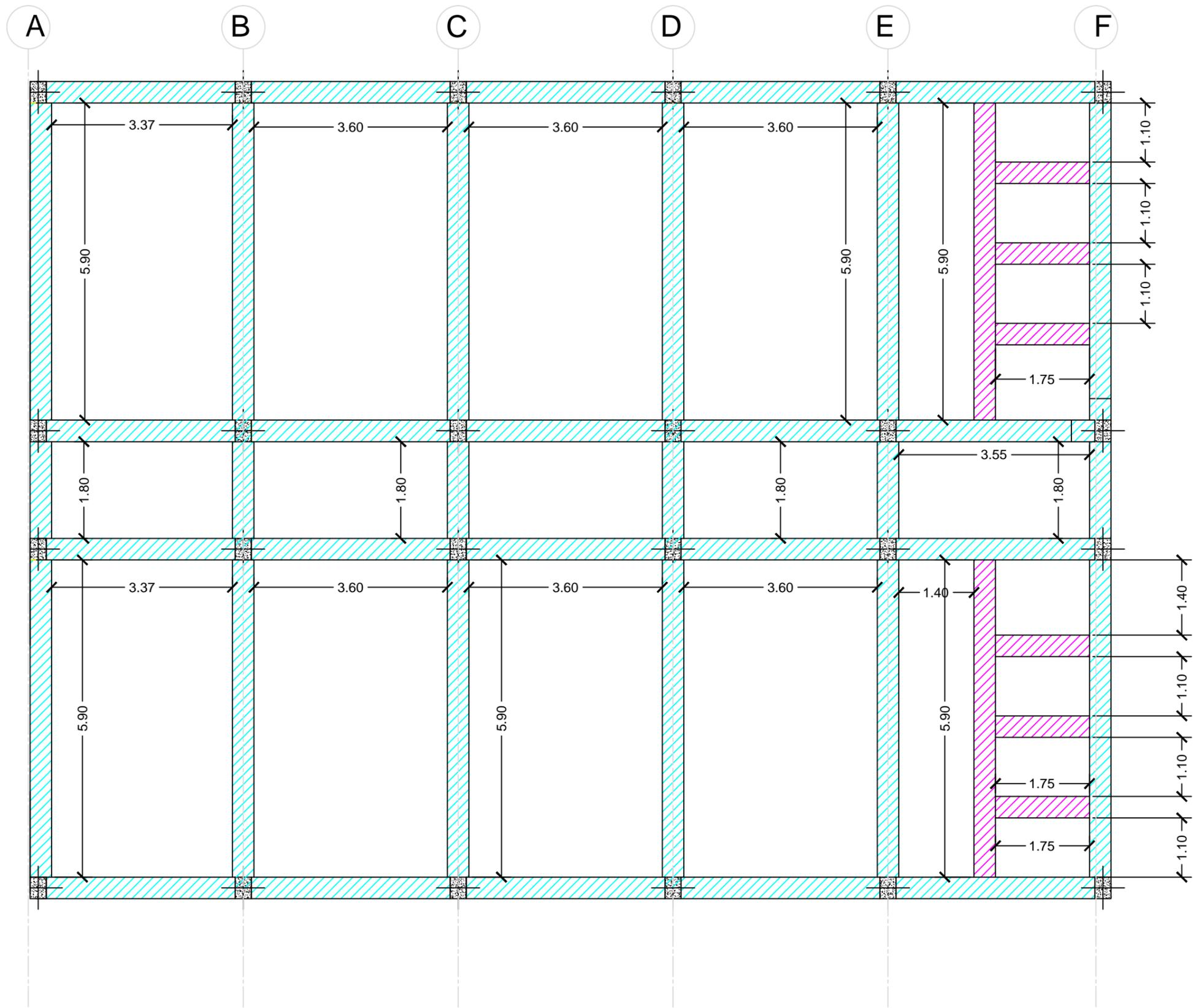
Layout for construction of backfilling materials for floor of open spaces #2 and 3 for new NIEC compound at aviazione gravel road of Mogadishu, Somalia.
