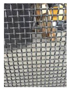
In this slot will be placed elements of 15x15 mm metal mesh and all its necessary accessories
