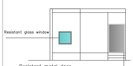
Resistant metal door, plates from each plate thickness 6 mm, according to the technical specifications
