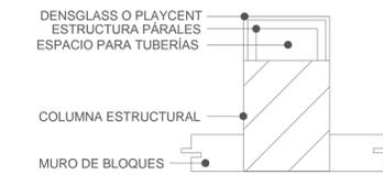
7 DETALLE COLUMNA ESTRUCTURAL CON COLUMNA FALSA
