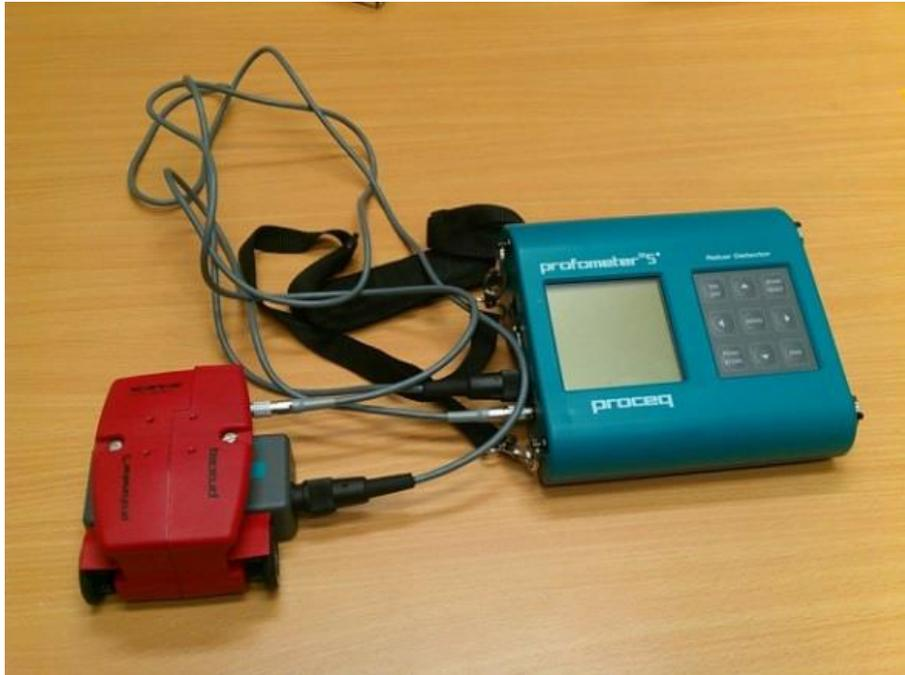
Imagen 5: Ferroscan PROFOMETER 5-PROCEQ.
