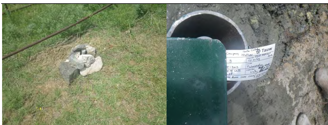
Figure 4.2 Left: Monitoring well 8, protected by rocks. Right: Monitoring well 9, protected with steel well head. All monitoring wells are equipped with weather proof labels providing details on the monitoring wells
