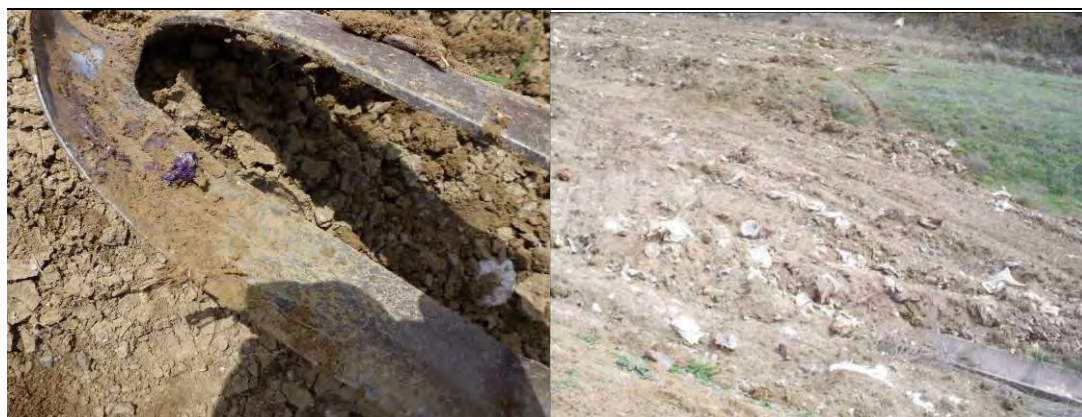
Figure 4.6 Left: pure product particle on auger head (likely Granosan) Right: The situation (April 2010) before closing of the landfill, with pesticide waste scattered around the current landfill body
