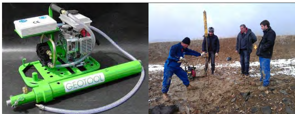
Figure 2.2 A Left the DCPT Geotool and right a DCPT measurement
