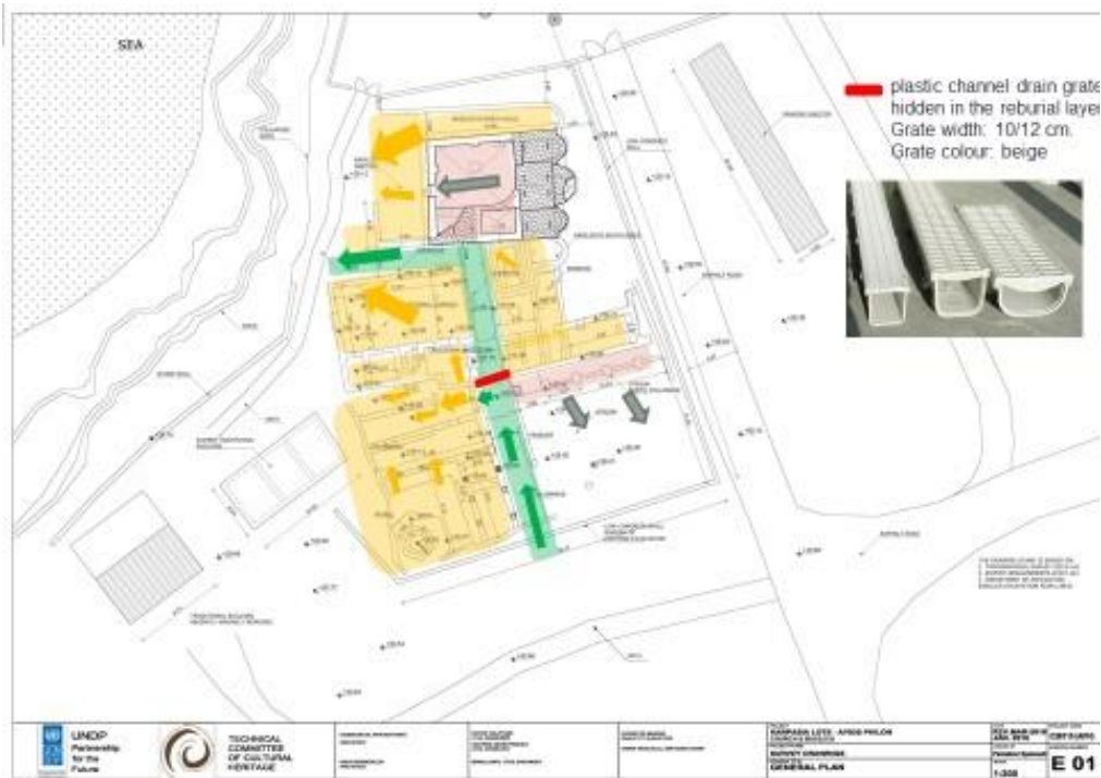
Pl. 1: Arrows show the reburials' inclinations for the rainwater management.
