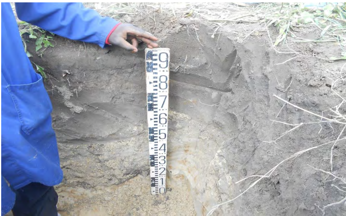
Figure 2 Dark grey overburden and next horizon of pit sand.
