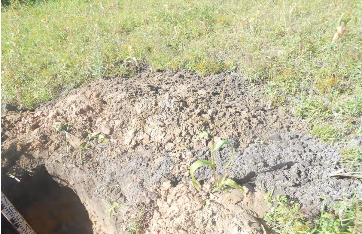
Figure 3 Pit sand as the 2nd horizon in trial pi no: 02
