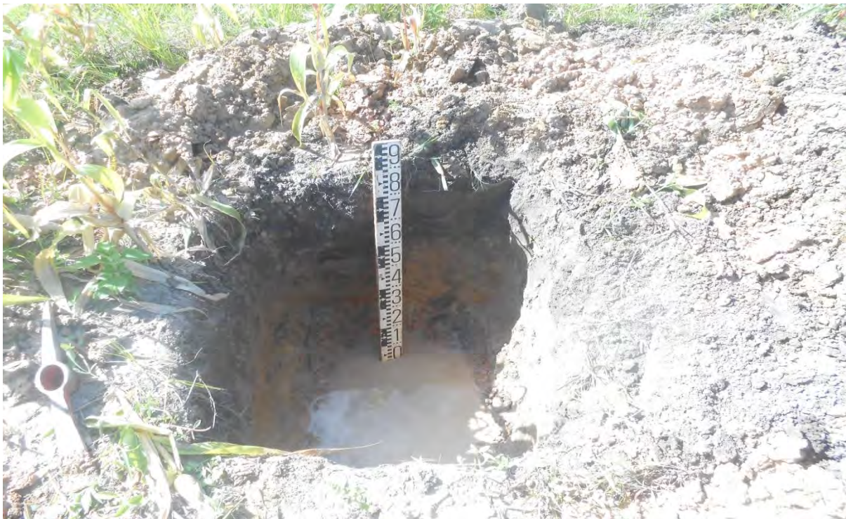
Figure 3 Pit sand as the 2nd horizon in trial pi no: 02
