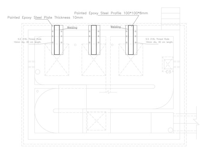
Pump Guide Holder For New Pumps Installation In PS2 & PS3
