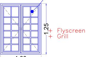
3" Rectangular H&V LEXAN @ DOOR LOEAF FINISHED OIL PAINTS 3COATS ON 3COATS OF ANTI-CORROGION PAINT 3HEAVY DUTY HINGES
