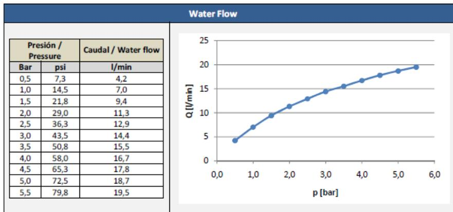
Figure 17 : Water flow for Mixer
