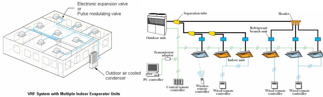
Figure 23 : VRV Installation Scheme
