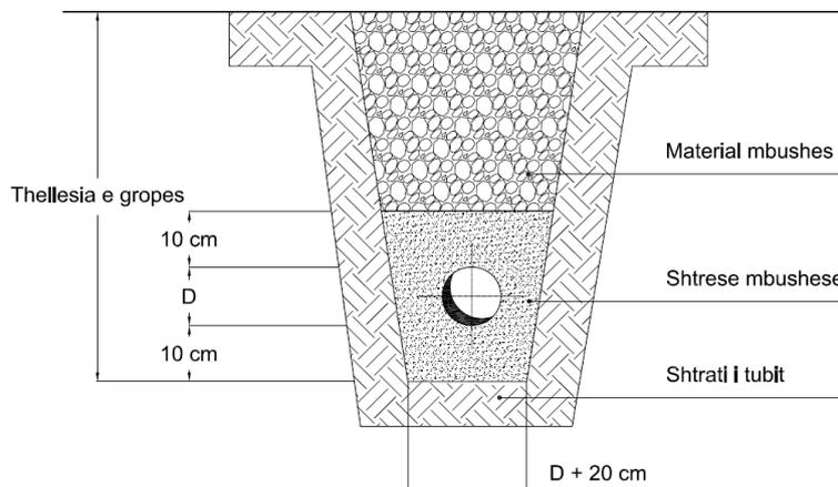
Figure 13 : Method of installation pipes
