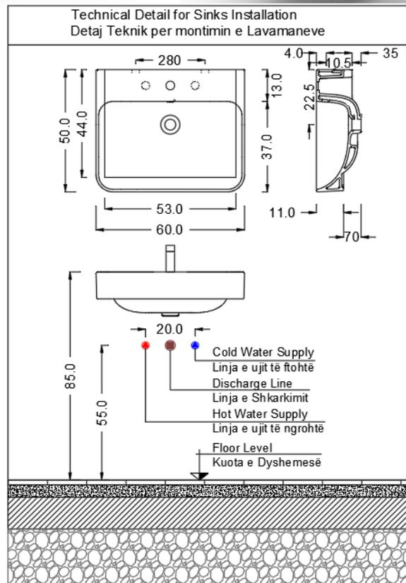
Figure 18 : Technical detail installation for Sink
