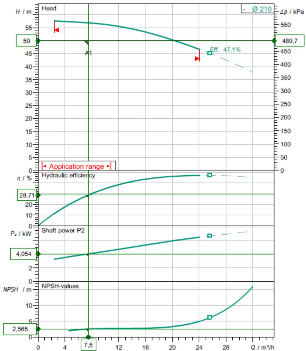
Figure 2 : Technical Data for Firefighting Pump
