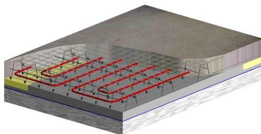
Figure 34 : Detail for underfloor heating installation
