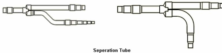
Figure 24 : Joint for separation pipes
