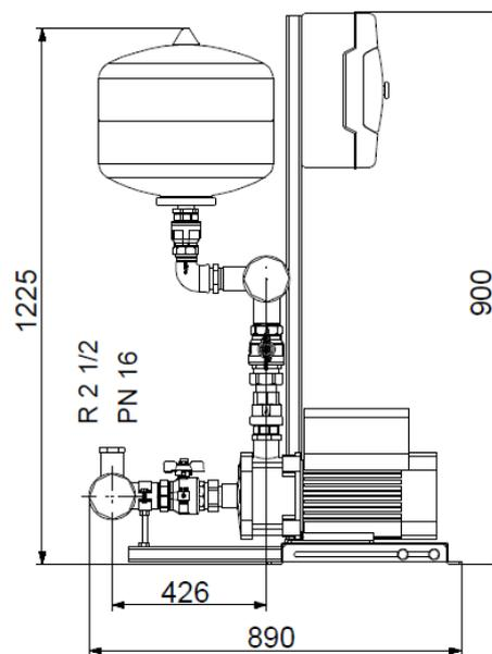
Figure 7 : Technical Data for Sanitary Water Pumps
