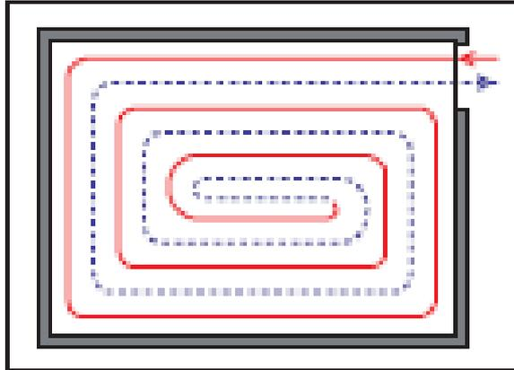
Figure 35 : Floor heating pipe assembly scheme
