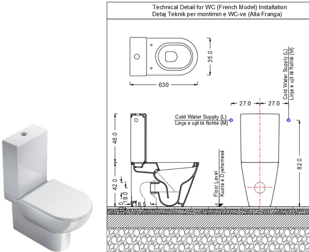
Figure 14 : Technical Detail for Toilets (French Model)
