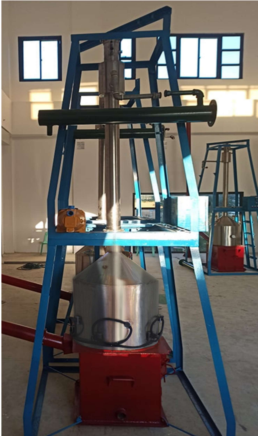
Picture of the Column & Kettle with imbedded electric heater
