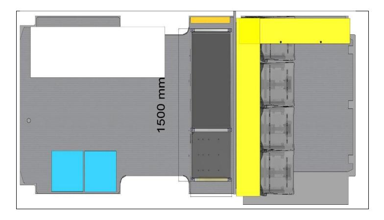
Description of the rack in the cargo compartment, which is used for storage and transportation of medical equipment.
