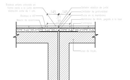
DETALLE JUNTA HORIZONTAL INTERNO EN PISO.
