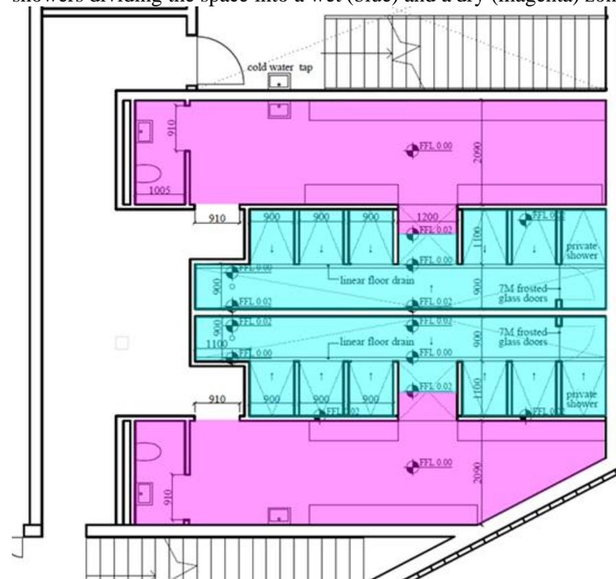
Figure 1 Plan of the proposed work for the changing rooms area
